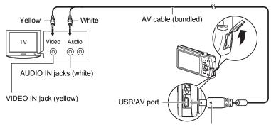
Making sure that the ◀ mark on the AV cable connector is towards the monitor screen side, connect the cable to the camera.
